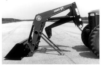
IMPORTANT: To avoid hydraulic hose damage, be alert and make sure hoses do not catch on tractor and/or loader during mounting or dismounting.
